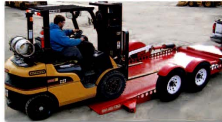
A flip of a switch hydraulically lowers the deck to ground height to allow fast, drive-on access.
