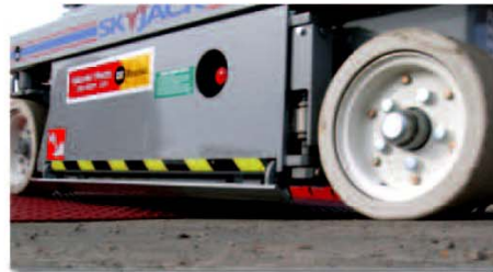
When lowered, the Lo Riser allows a minimum 5° angle ideal for low ground clearance or reduced gradeability vehicles.
