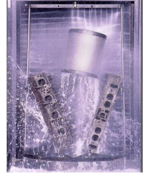
360° spray flow and 0° jets washes parts cleaner and faster!
